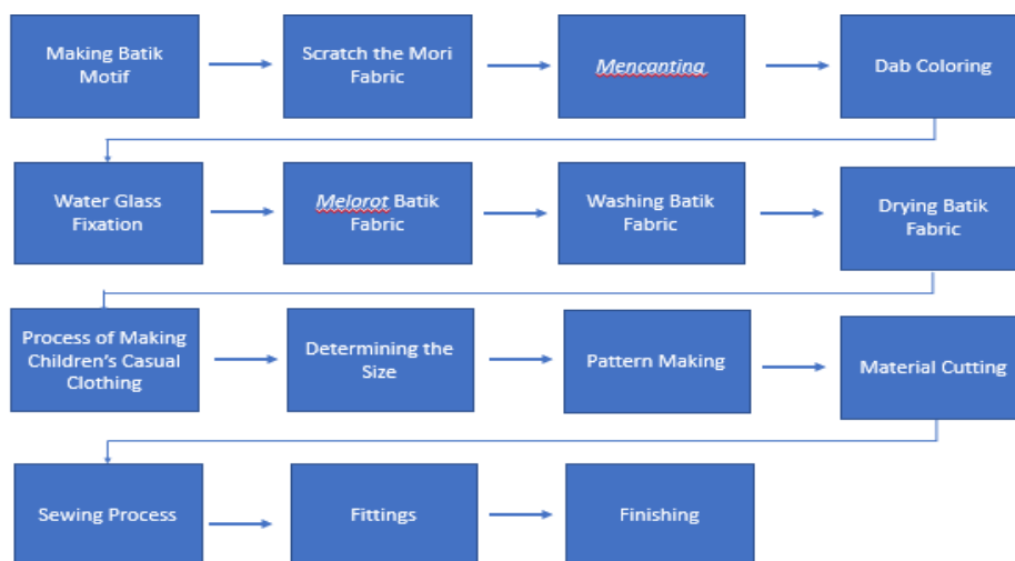
Picture 3. Line of Work
