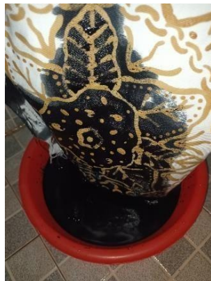
Picture 9. Coloring cloth jeans use remasol black NN
