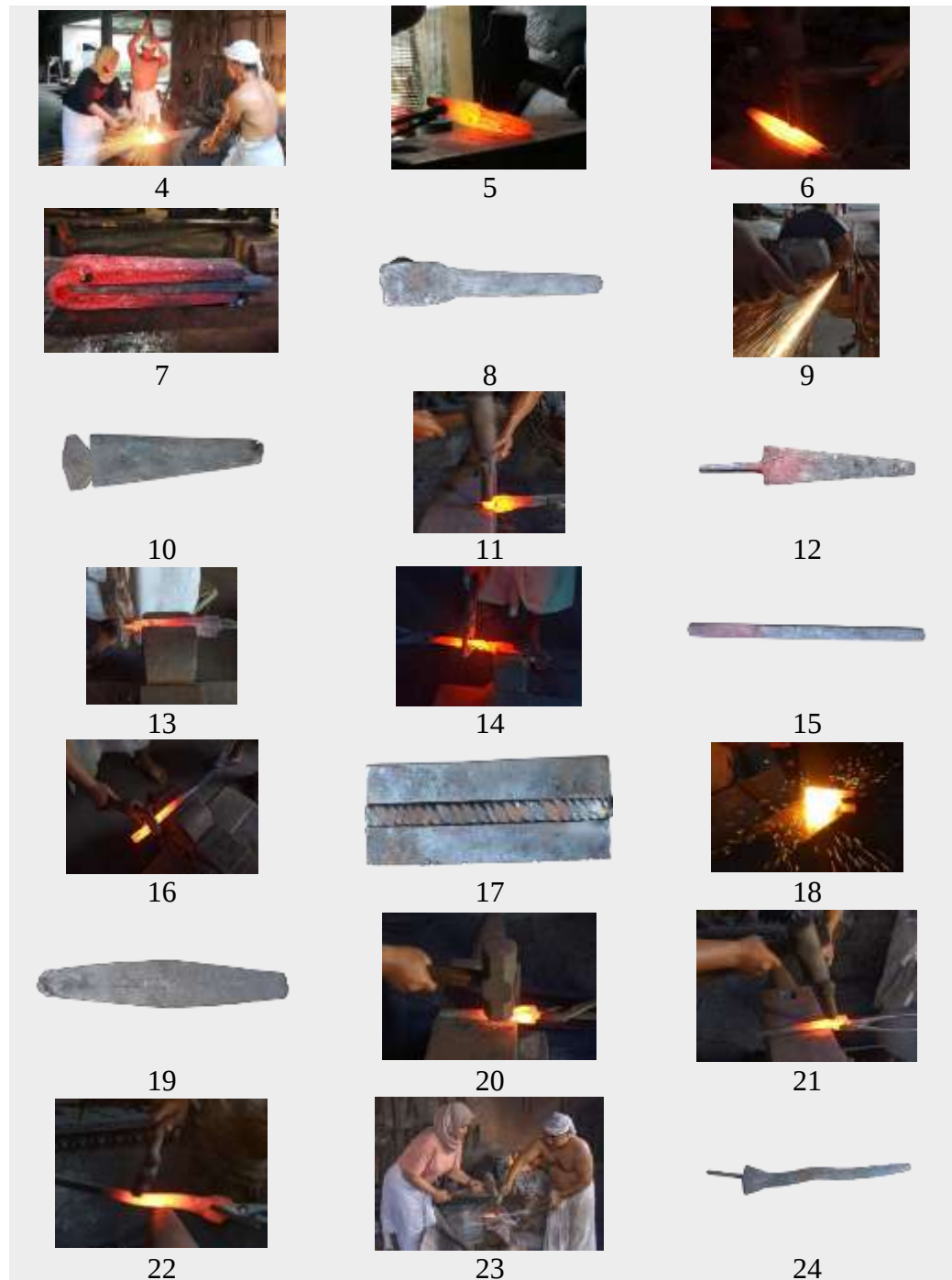
Figure 11. Process of keris forging (Photo: Puput Saputri, 2021)
