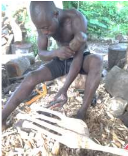
Figure 51. Master wood carver detailing with chisel (Photo: Agyei et al)
