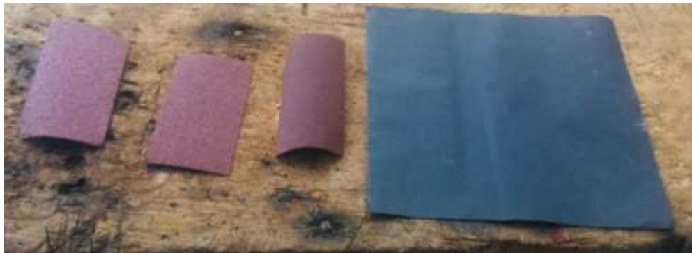
Figure 27. Sand paper of 60, 80, 120 & 240 grit (Photo: Agyei et all.)
