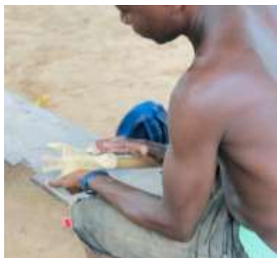
Figure 57. Master wood carver sanding wooden sculpture from coarse to fine (Photo: Agyei et al)
