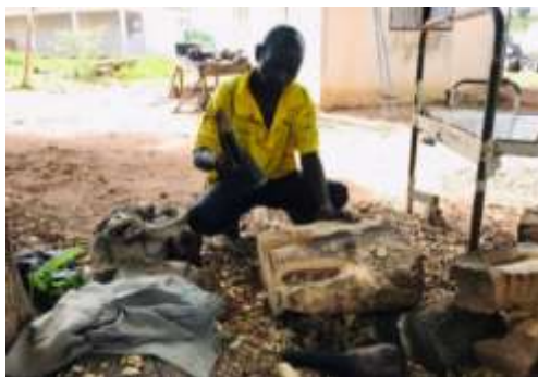
Figure 19. Master wood carver blocking out with adze ('U' shaped) (Photo: Agyei et al.)
