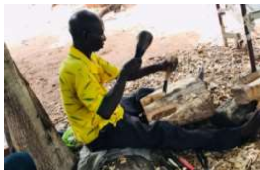
Figure 20. Master wood carver blocking out with large sized 'C' gouge (Photo: Agyei et al.)
