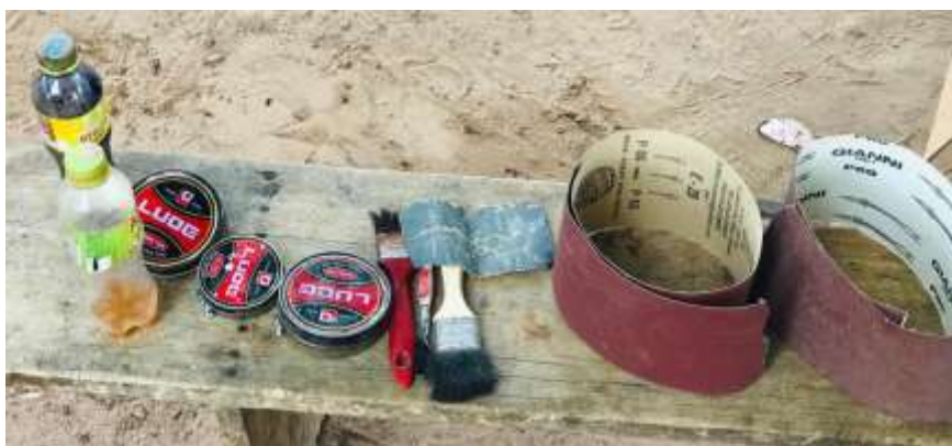
Figure 54. Sand paper (60, 80, 150 and 400 grit), brushes, wax polish (brown, black and neutral) kerosene and diluted potassium permanganate (Photo: Agyei et al)
