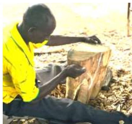
Figure 22. Master wood carver using chalk to mark features (Photo: Agyei et all.)
