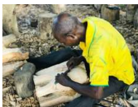
Figure 24. Master wood carver using spoke shave to whittle (Photo: Agyei et all.)
