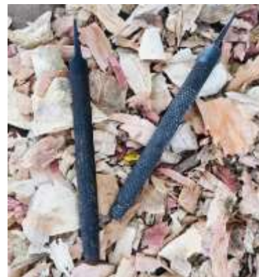
Figure 11. Half rounded files (rough and soft) (Photo: Agyei et al.)
