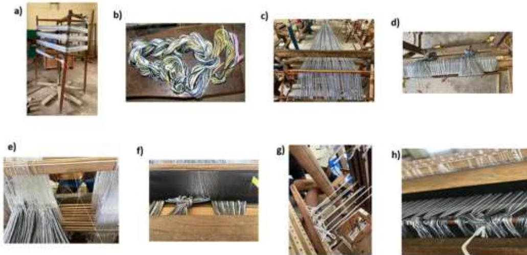
Figure 2. a) Milling, b) Chaining, c) Raddling, d) Beaming (Completed), e) Heddlng, f) Denting/Reeding, g) Shaft-treadle tie-up, h) Warp ends-cloth beam tie-up
