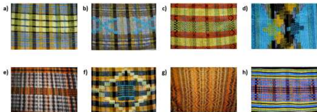
Figure 4. Woven Samples - a) plain weave, check effect (normal spun yarn, and flash yarn), b) hand-picking effect (knit yarn and normal spun yarn), c) simple twill weave, and akyem design effect (flash yarn, metallic yarn and normal spun yarn), d) plain weave and handpicking effect (knit yarn and normal spun yarn), e) Basket weave effect, (nylon cord and normal spun yarn), f) plain
