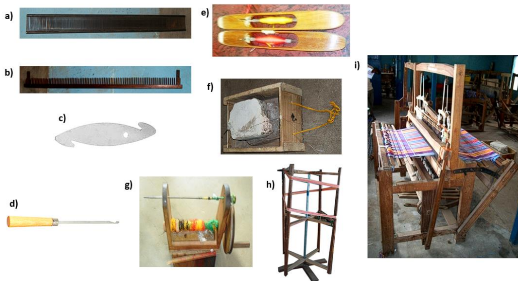
Figure 2. Broadloom and selected weaving accessories: a) reed, b) raddle, c) reed hook, d) heddling hook, e) shuttles, f) drag box, g) bobbin winder, h) warping mill, i) broadloom (Source: Author's Shot, 2025)
