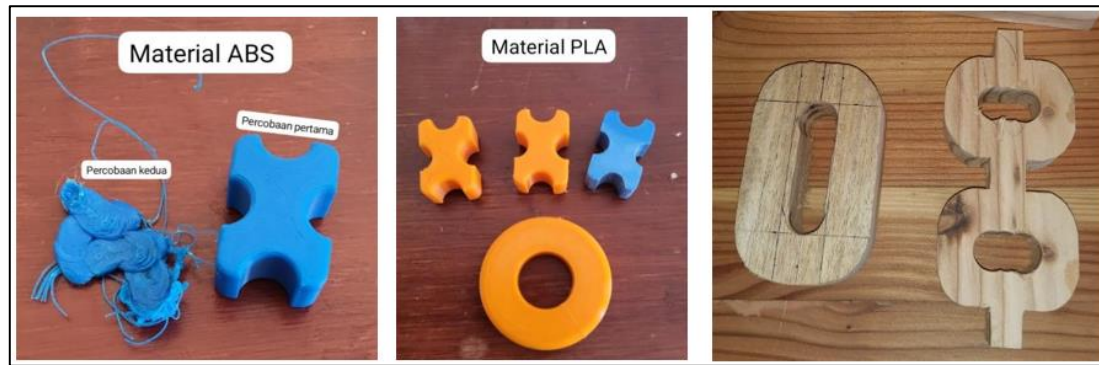
Fig. 7. Material Exploration of ABS, PLA, and Wood for Prototype Development
