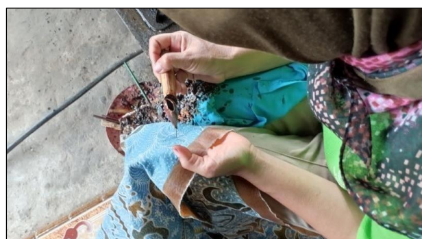
Fig. 3. Hot Wex Attachment Process ( malam ) Using Canting
