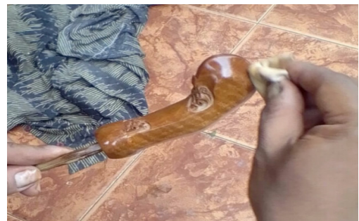
Gambar: Proses finishing hulu (Foto dan scan: Ari Harmawan: 18/12/2018)
