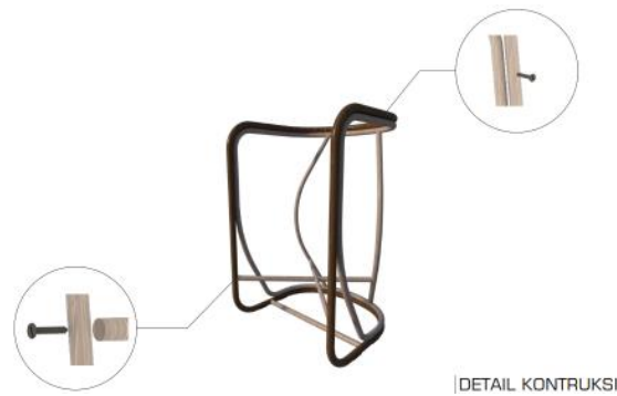
Fig. 23. Construction of the therapist chair, joints using screws 5 cm
