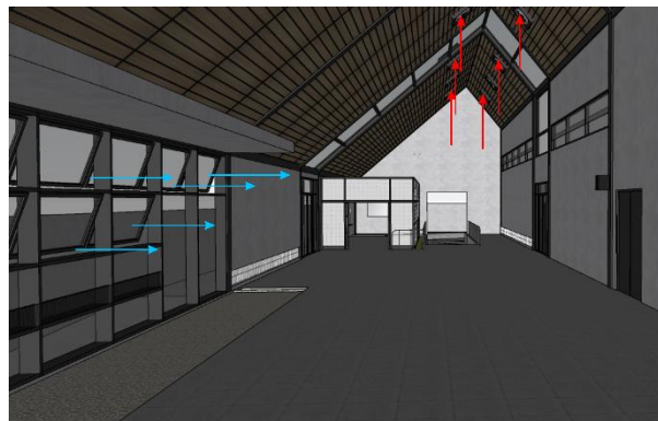
Fig 4. Implementation of Turbine Ventilators at AGHE Coffee & Resto
