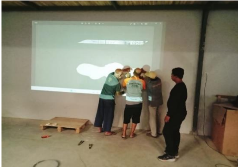
Fig. 9. The weaving process of the frame using the projection of 1:1 scale images as a guide (Personal Documentation)
